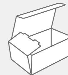
Fefco style 0421 Folding box with locking sides
